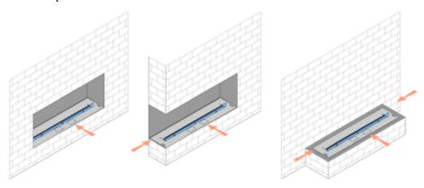
Situations in which installation of a glass shield is forbidden:
