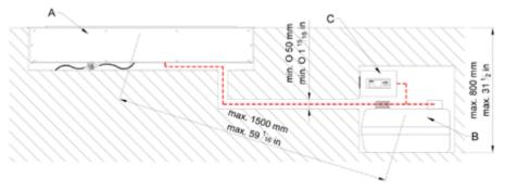
Make a cavity for the appliance following the diagram below. Ensure that the plane within the cavity on which the appliance is to be installed is level.
