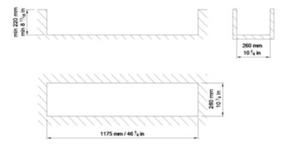
The difference in level between the ends of the appliance must not exceed 2mm. Poor levelling may cause abnormal operation of the appliance and, in extreme cases, it can cause leaks of the bio-ethanol fuel and the danger of fire.
