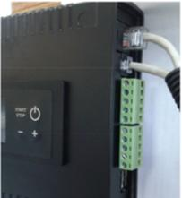
Then connect the cable supplied with a connection block at the end of the cord. Note that connection to the mains must be made by a qualified electrician.
