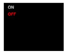
Using "+" button choose OFF option and confirm with "-" button. The device automatically returns to main display and 'Fast start' function will be turned off.
