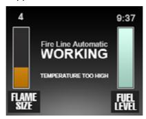
If the temperature of the device still increases, the device will switch off. When the temperature decreases to a safe level, flame size can be increased again.
