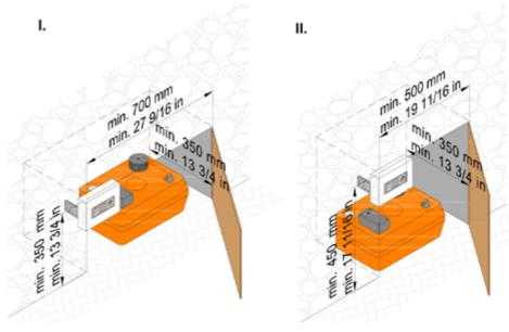
Place the external tank 'B' in the cavity and install external control panel 'C'. In order to install the control panel use four screws 'D' or two wall plugs 'E' (depending on the material).
