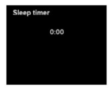
Using "+" button choose the desired time (not longer than 3 hours) and confirm with "-" button.
