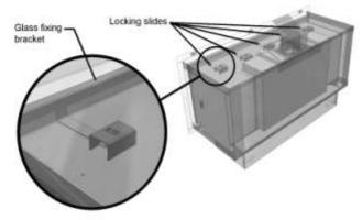
Refit the 3 hex screws located at the bottom of the glass fixing (see fig. 105). Care must be taken when using the allen key to prevent damage to paintwork. Fig. 105
