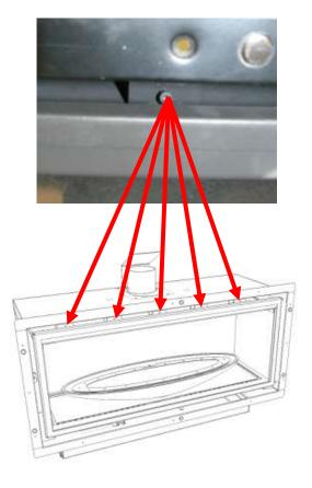
Remove the 3 hex screws located at the bottom of the glass fixing (see fig. 26).
