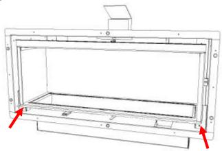
Remove the screws to release the inner casing from the outer casing (see fig. 48)
