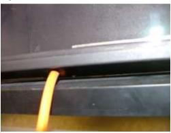
Ensure the wiring is away from the burner base and making sure no wiring is trapped inbetween any metal work.
