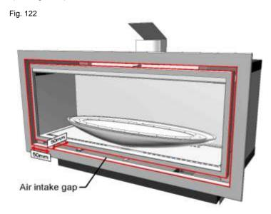
If the appliance and chimney is functioning correctly all smoke should be drawn into the air intake and out of the room.
