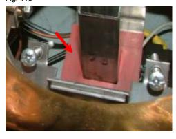
Fit the burner and secure using the securing/ levelling screws. To level the burner screw in the left or right screw further. (Fig. 116, 117)
