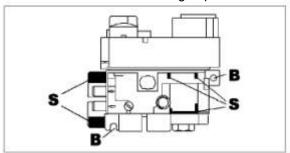
Fig. M3: S=Clamp Areas, B=Mounting Points
