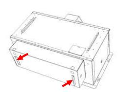
Fit the outer casing in the opening and secure (see fig. 58-60). There is no need to use all securing points.
