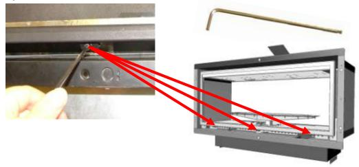
Tighten the five glass fixings at the top using the 4mm ball head allen key hexagon key. Care must be taken when using the allen key to prevent damage to paintwork. (see fig. 106).
