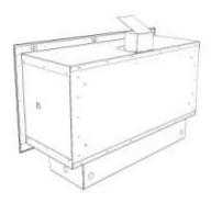
Undo the five glass fixings at the top using the 4mm ball head allen key supplied (see fig. 25)
