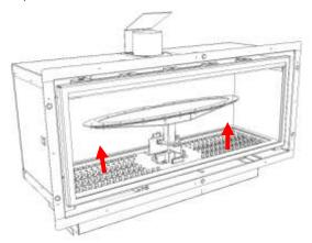
Lift the burner base assembly to access the wiring.
