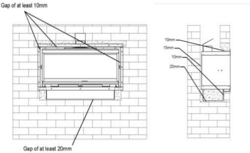
Make sure that the appliance is not carrying the weight of the chimney breast.
