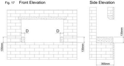
The front filling is approx. Height 110mm x Depth 70mm including plaster and skimming (see fig.18)
