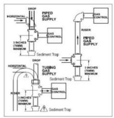
Fig. M2: Sediment Trap (where required)
