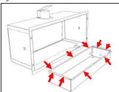
Remove the screws attaching the spigot and drop the spigot out (see fig. 52, 53).
