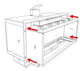
When sliding the inner casing it is important to ensure the spigot slides into the channels to form a good seal (see fig. 68, 69)
