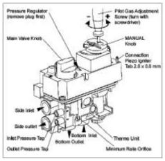
Fig.M4: Combination Control GV60, Connections and Adjustment Options
