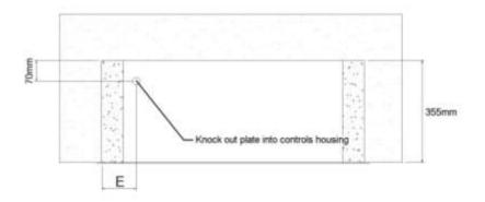
If routed through the back of the appliance the position of the knock out plate is shown in fig. 20. (For measurement 'E' See table on page 10)
