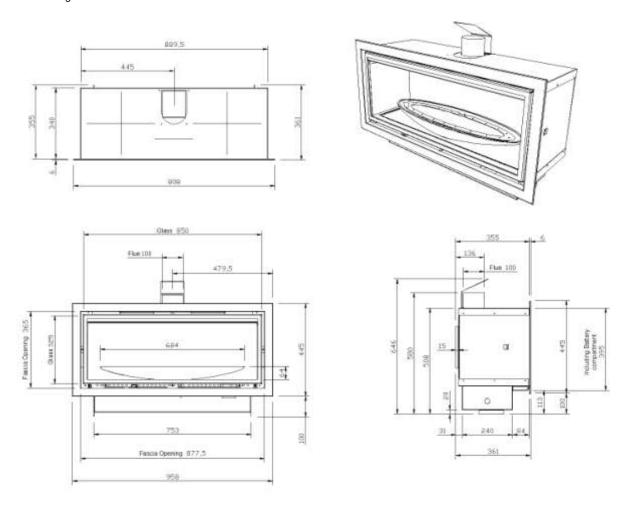
IMPORTANT NOTE – Allowances must be made for the battery compartment
