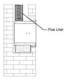
If the appliance is fitted with a flue liner the debris shield will not be required (see fig.14).
