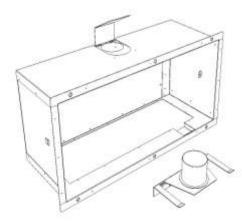
Remove the screws holding the debris shield and drop the shield out (see fig. 54, 55).
