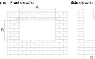
The appliance supports are approx. (For measurement 'D' See table above) Height 135mm x Depth 355mm (Including plaster and skimming) (see fig.17)
