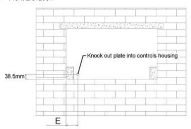
Note – This appliance must not be used as part of the wall support structure.
