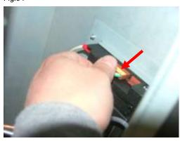
Refit the wiring / black grommet into the interrupter block and tighten the interrupter nut, ensure the lever tip is fitted so when pushed down the lever connects with the rest button (See fig. 95-98) check all wiring is connected then connect the battery lead, a long beep will be heard (see fig. 98).
