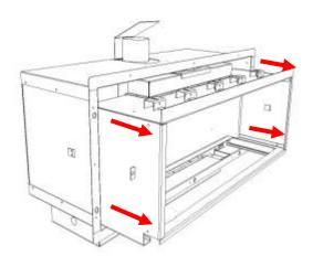
Place the outer casing on its back and remove the screws holding the controls housing then remove the housing (see fig. 50, 51).
