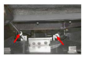
Carefully lift the burner from the appliance. NOTE – The burner bed fibre matting used to spread the flame can irritate the skin when handled and is advised to wear protective clothing. The fibre matting is also very fragile and must be handled with care to avoid damage. IMPORTANT – Only use a soft brush to clean the surface. Do NOT use a vacuum to clean the fibre bed (see fig. 29).
