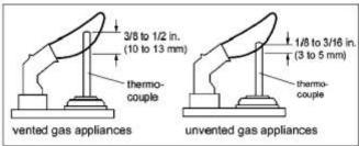
Fig.M5: Proper Flame Impingement on thermocouple
