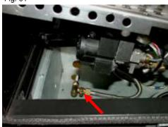
Reconnect the spark lead cable and 8 core cable. (See fig. 92-94). Fig. 92  $\,$  Fig. 93  $\,$
