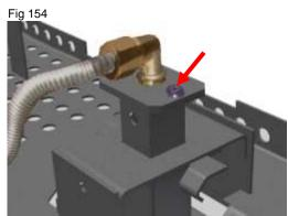
Remove the injector nut using a 13mm spanner (see fig. 155). NG Elbow Injector has a single hole markings are located on the nozzle (see fig. 156)
