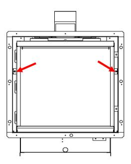
Carefully slide the inner casing out (see fig. 37)
