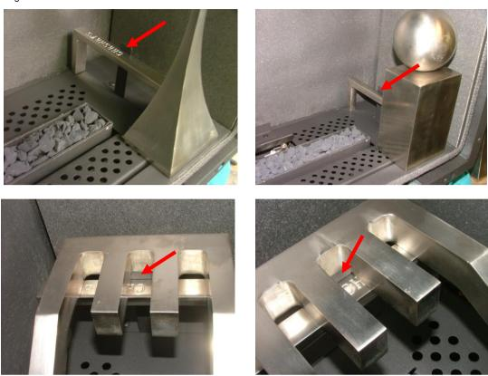
Slide the centre front bracket in place and screw down. (See fig. 75)
