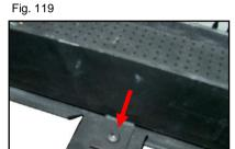
Lift the burner and attached injector / flexi tube. Disconnect the flexi tube using a 15mm spanner and remove the 2 screws to release the injector and bracket. (see fig. 120)
