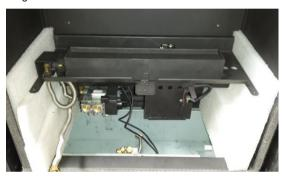
Connect the burner inlet tube to the isolation valve / pressure test point (see fig. 60), fit the on /off switch (see fig. 61) then remove the support foams by sliding out, then drop the burner assembly into the controls housing.
