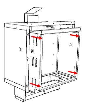
Place the outer casing on its back and remove the screws holding the controls housing then remove the housing (see fig. 38).
