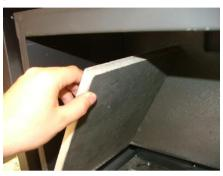
Remove the panel bracket and screw on the opposite side (mirror image of fig. 126), lift the side panel out (see fig. 127) hold back the back panel at the same time to ensure it doesn't fall. (see fig. 128)
