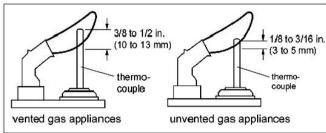
Fig.M5: Proper Flame Impingement on thermocouple
