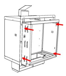
When sliding the inner casing it is important to ensure the spigot slides into the channels to form a good seal (see fig. 51)
