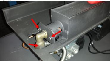
Remove the injector nut holding the bracket using a 13mm spanner.
