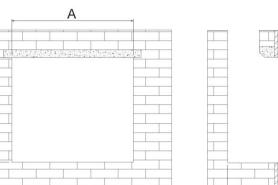
The appliance supports are approx. (For measurement 'D' See table above) Height 135mm x Depth 355mm (Including plaster and skimming) (see fig.21)
