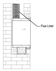
If the appliance is fitted with a flue liner the debris shield will not be required (see fig.18).
