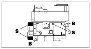
Fig. M3: S=Clamp Areas, B=Mounting Points
