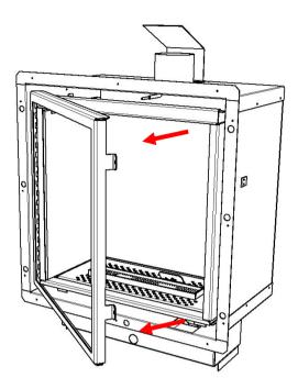
The door can be removed by lifting the door and carefully sliding the door out of the slots located on the left side of the appliance. (see fig. 32)
