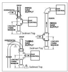
Fig. M2: Sediment Trap (where required)
