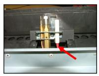
Undo the 4mm pipe with a 10mm spanner (see fig. 111) and disconnect from the pilot. Remove the bracket (see fig. 112).
