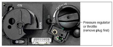
Fig.M6: Combination Control GV60, Cover
