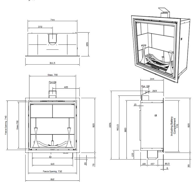
IMPORTANT NOTE – Allowances must be made for the battery compartment
