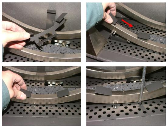
Place log 1 so that the knuckle is sat on the burner ridge, note the position of the log to the pilot. (See fig. 76)
