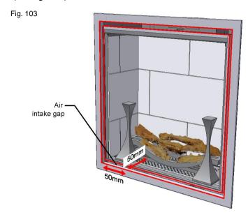
If the appliance and chimney is functioning correctly all smoke should be drawn into the air intake and out of the room.
