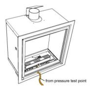
Ensure the wiring is away from the burner making sure no wiring is trapped in-between. At this point test the connections for soundness.
