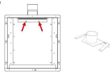
Remove the screws holding the debris shield and drop the shield out (see fig. 40).
