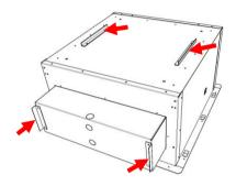
Fit the outer casing in the opening and secure (see fig. 42). There is no need to use all securing points.
