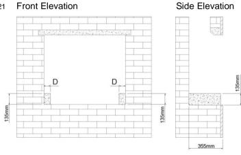
The front filling is approx. Height 110mm x Depth 70mm including plaster and skimming (see fig.22)
