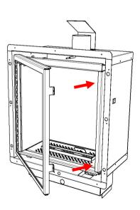
Refit the 2 hex screws (see fig. 65). Care must be taken when using the allen key to prevent damage to paintwork.
