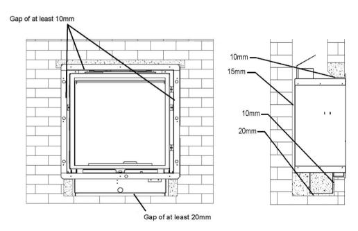
Make sure that the appliance is not carrying the weight of the chimney breast.
