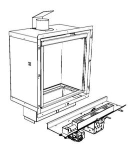
Remove the screws to release the inner casing from the outer casing (see fig. 36)
