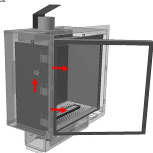
Remove the log base to access the burner assembly (see fig. 33).
