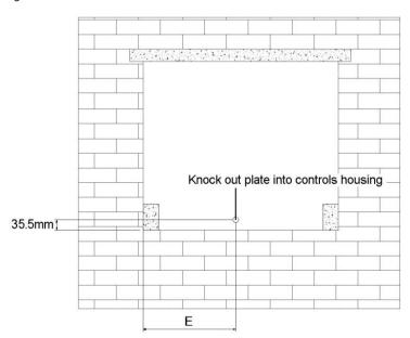
Note – This appliance must not be used as part of the wall support structure.
