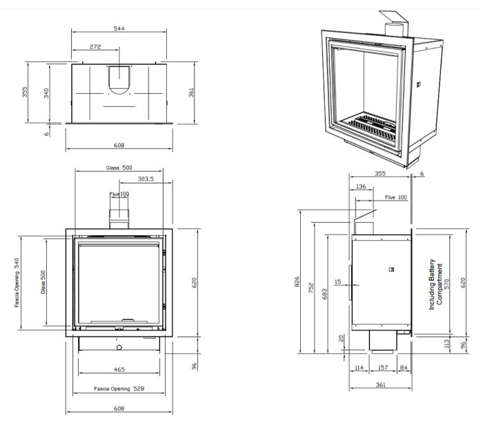
IMPORTANT NOTE - Allowances must be made for the battery compartment
