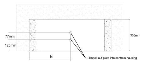
If routed through the back of the appliance the position of the knock out plate is shown in fig. 24. (For measurement 'E' See table on page 10)
