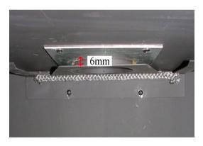
Slide the inner casing into the outer casing (see fig. 50)
