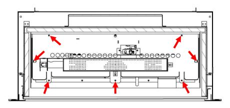
Carefully lift the burner assembly and control system from the appliance. (See fig. 35)
