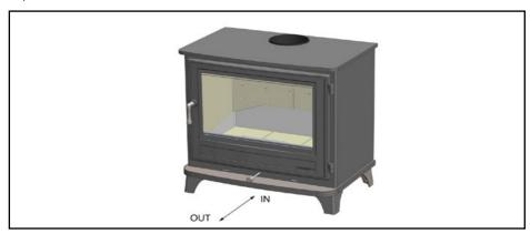
With the air control bar fully out the maximum air is entering the stove at the top front (air wash) and through the rear bricks. When the air control bar is pushed in the air is reduced proportionally between the air wash and the rear brick to give the best "burn". When the air control bar is fully in there is still air entering the stove via the air wash. Before lighting the stove ensure the baffle by-pass is free to operate.
