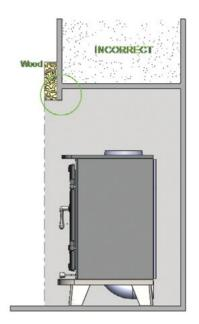
The closure plate must be fitted in such a away it does not allow the build up heat in the fire chamber i.e. flush as shown, the stove must also be in line or protruding forward beyond the fire chamber. The regulations governing connecting flue pipes must be adhered to.
