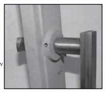
For adjustments on the hinge side of the stove the door must be removed. Lift the top off the stove, twist and rest on the fire cube. Open the door (Shoreditch, Shipton, Salisbury and Beaumont models) and lift from the hinge pins.
