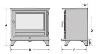
Soft furnishings should be at least 1000mm from the appliance. Distances to combustibles: Rear: 500mm (400mm for 12WS), Sides: 350mm
