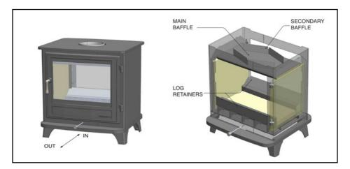
With the air control bar fully out the maximum air is entering the stove at the top (preheated air wash) and at the base of the firebox. When the air control bar is pushed in the air is reduced proportionally between the air wash and base of the firebox to achieve the best "burn". When the air control bar is fully in there is still a small amount of air entering the stove via the air wash.
