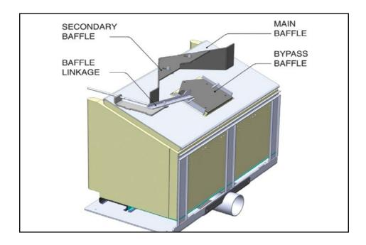
The secondary baffle is secured to the top underside of the stove using the slots provided. It is removed by sliding to the rear of the stove.
